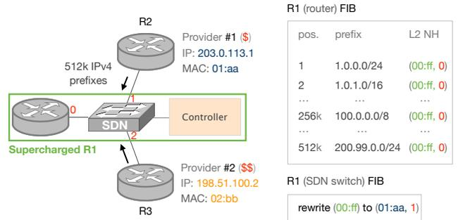
Figure 2: In a supercharged router, the combined FIB is hierarchical, each FIB entry in the router points to a virtual L2 NH or pointer that is resolved in the SDN switch. Upon failure of  $R2$ , only *one entry*—the pointer value—needs to update to restore full connectivity.
