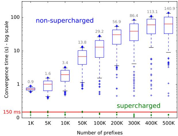
Figure 5: With respect to the normal convergence time which increases linearly with the number of prefixes, our supercharged router *systematically converged within 150ms*. In contrast, the non-supercharged router took more than 2 minutes to converge in the worst-case.
