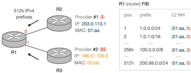
Figure 1: In a classical router, the Forwarding Information Base (FIB) is flat, meaning each entry points to the actual physical L2 NH. Upon a failure of  $R2$ , every single entry (512k) has to be updated to restore full connectivity, a time-consuming operation.
