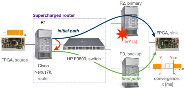
Figure 4: Overview of our HW-based convergence lab.  $R2$  is rendered inaccessible, causing  $R1$  to switch to  $R3$  for every single prefixes. At the same time, we use FPGAs to precisely ( $\mu$ s resolution) measure the convergence time. Ultimately, we compare the convergence time of the supercharged  $R1$  and the standalone  $R1$ .
