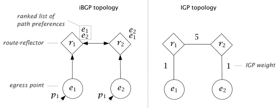
**Figure 5.1** Graphical notations used in the thesis when referring to an iBGP configuration
