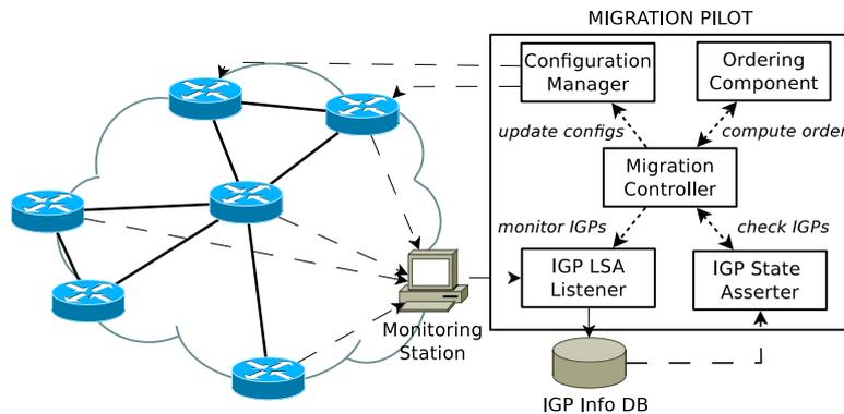
**Figure 3.9** Design of the provisioning system. The provisioning system automates all the reconfiguration process. It computes the ordering, monitors the network and pushes the intermediate configurations in the appropriate order.
